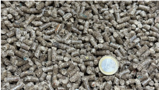
Waste Wood Pellets Shrinkage start temp 980-1080°C
